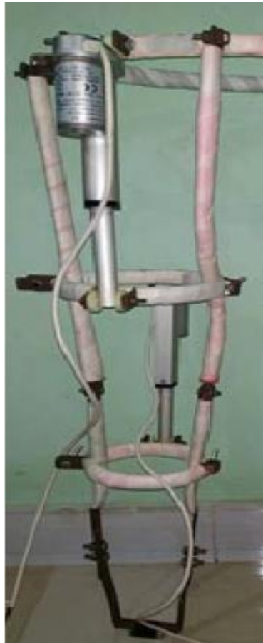
Fig .11 Lower Limb Exoskeleton with Linear Actuator
