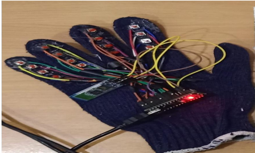
Fig 5.1 Glove Fitted with Buttons and Arduino
