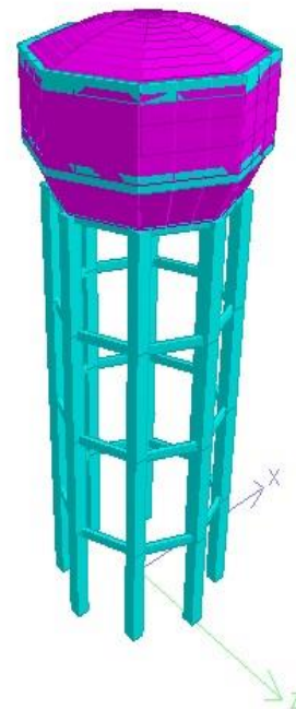
Fig 3 Framed Type model prepared in Staad-Pro
