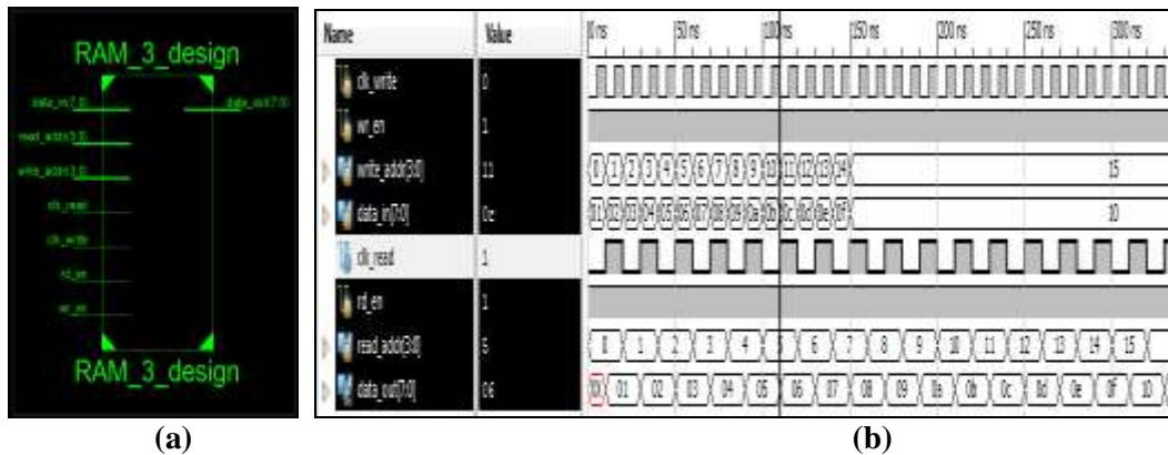
Figure 4. (a) RTL schematic of DPRAM and (b) Simulation waveform of DPRAM.
